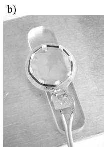
Fig. 5. The axial distance dependency of the coupling coefficient between the coils. The coil L_1 (120 mm diameter) is considered as the primary winding. a) The secondary coil (30 mm diameter) is measured in the free space or with a parallel metal plate below the coil in the distances of 3 mm and 13 mm (the metal plate is on the outer side – not between the coils); b) the secondary coil above the large metal plate in the distance defined by the ceramic pad.
