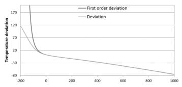
Fig. 3. Comparison of the calculated temperature deviation due to size of source effect for direct reading thermometers (4) and the one obtained by the first order approximation for thermometers with the electrical output signal (8). The room temperature was assumed to be 21°C.
