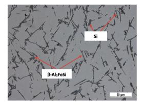
Fig. 5. Morphology of eutectic silicon in AlSi7Mg0.3 alloy with 1.2 wt. % Fe and 0.1 wt. % Mn (sample C1)
