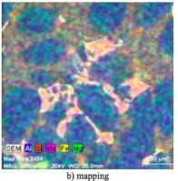
Fig. 4. Mapping of Al<sub>15</sub>(FeMn)<sub>3</sub>Si<sub>2</sub> phase in the AlSi7Mg0,3 alloy with 0.8 wt. % Fe after adding 0.6 wt. Mn (sample B4)
