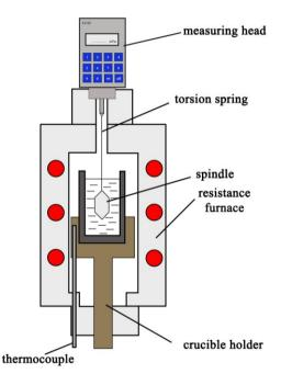
Fig. 3. Diagram of a rotating-cylinder viscometer
