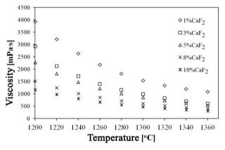
Fig. 5. Influence of added CaF2 on viscosity of decopperised slag
