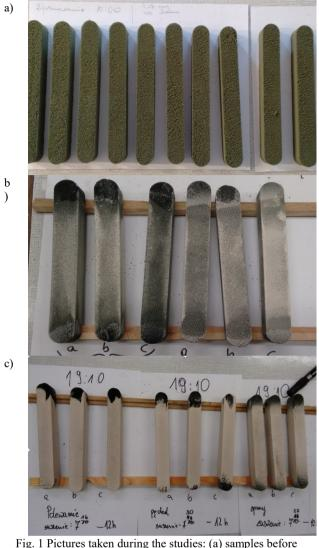
application of coating, (b) after application of penetration layer, (c) after coating application
