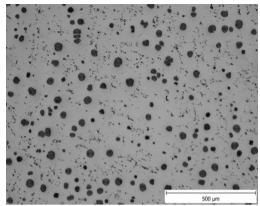
Fig. 13. Metallography of sample D – Axis, mag. 100x
