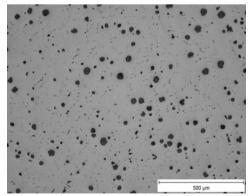
Fig. 7. Metallography of sample A – Edge, mag. 100x
