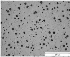
Fig. 8 Metallography of sample B - Axis, mag. 100x
