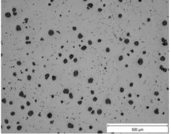
Fig. 9. Metallography of sample B – Edge, mag. 100x
