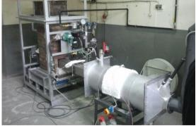
Fig. 1. View of the research stand for the thermal utilisation of post-reclamation dusts: in the stage of testing operations in the final version
