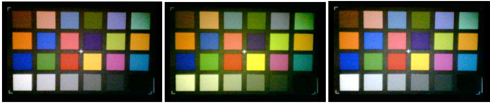
Fig. 17. Comparison of the image of the colour chart illuminated with: on the left – a multi-emitter source with CCT = 5500 K; in the middle – a phosphor-converting white LED with CCT = 6000 K; on the right – a multi-emitter source with CCT = 6500 K.
