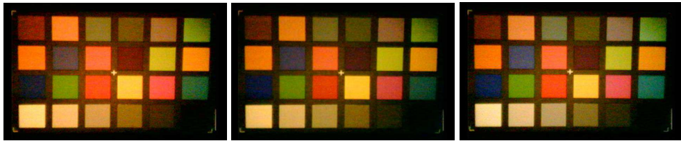
Fig. 18. Comparison of the image of the colour chart illuminated with: on the left – a multi-emitter source with CCT = 2856 K; in the middle – a phosphor-converting white LED with CCT = 3300 K; on the right – a multi-emitter source with CCT = 3500 K.
