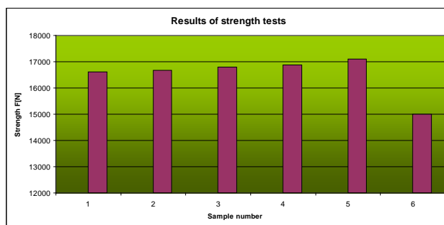
Fig. 4. The diagram of the details strength for various circulating scrap proportions
