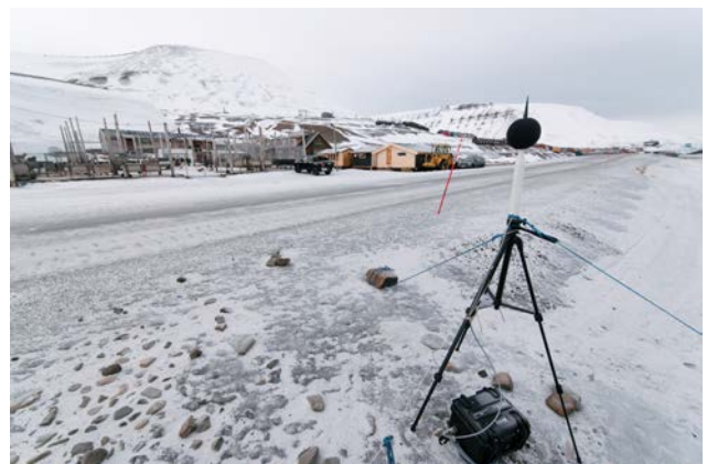
Fig. 10. A photo of a measuring point located between the road and main snowmobile route in Adventdalen (fot. Maciej Bernas).
