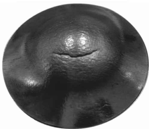
Fig. 7. Appearance of draw area after Erichsen test
