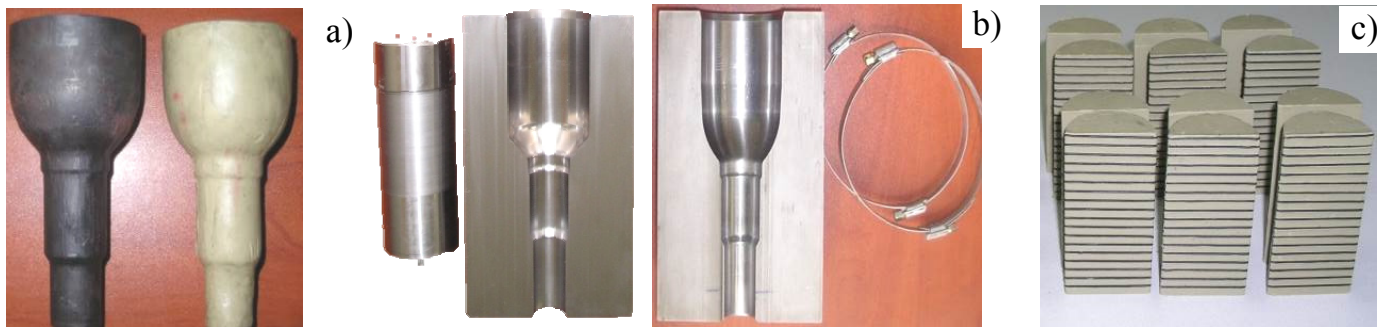
Fig. 2. a) Comparison of a forging made of steel after II extrusion operation with a forging made of filia wax, b) a tool set: a punch, two matrix halves, tightening belts, c) preforms made of modelling materials with horizontal flow lines
