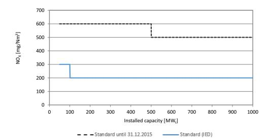
Fig. 2.  $NO_x$  emission standards for hard coal-fired plants (Directive 2010)
