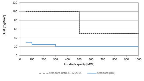
Fig. 3. Dust emission standards for hard coal-fired plants (Directive 2010)
