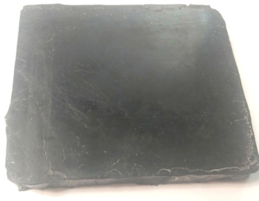
Fig. 2. Fabricated MWCNT reinforced epoxy nanocomposite sample
