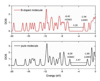
**Fig. 4.** DOS for 5,5'-Dibromo-2,2'-bithiophene and B-doped 5,5'-Dibromo-2,2'-bithiophene molecules.
