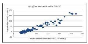
Fig. 2. Residual scatter plot of the EC2 compliance function J (t, t<sub>0</sub>) for concrete with water reducer (WR), silica fume (SF) and WR and SF (WR + SF) added simultaneously to the mix composition.
