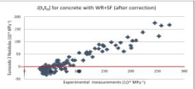
Fig. 5 Residual scatter plot of the EC2 compliance function J (t, t<sub>0</sub>) for concrete with Water reducer and Silica fume (WR+SF) before and after applying the correction coefficient.
