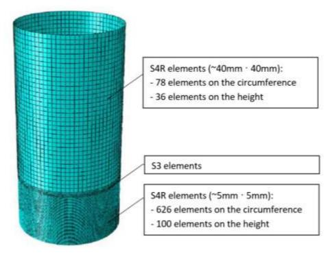
Fig. 4. Diagram of the adopted finite element mesh.
