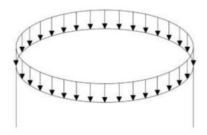
Fig. 2. Shell load diagram.
