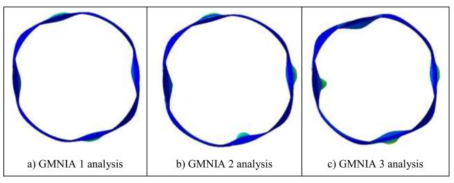
Fig. 12. Forms of loss of stability for GMNIA analyses.
