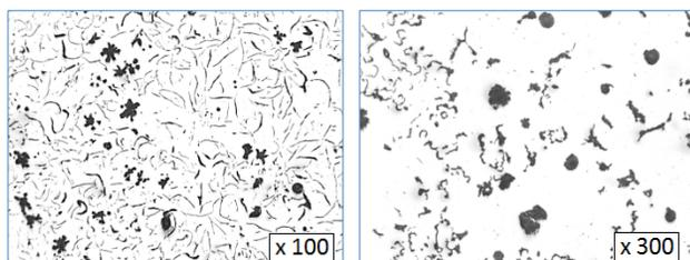
Fig. 10. Microstructure of bar sample Z5
