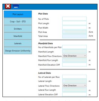
Fig. 2. The main program interface of Emission Uniformity on Sloping Surfaces (EUSS) model; source: own elaboration
