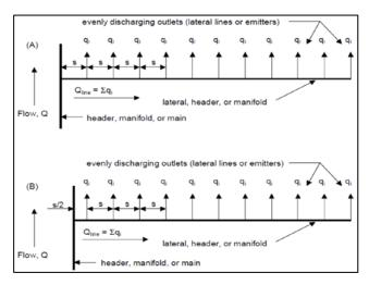
Fig. 6. Discharging outlet orientation for the multiple outlet factor: A = case of full space, B = case of half space; source: own elaboration
