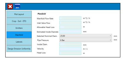
Fig. 7. Interface for Manifold design; source: own elaboration
