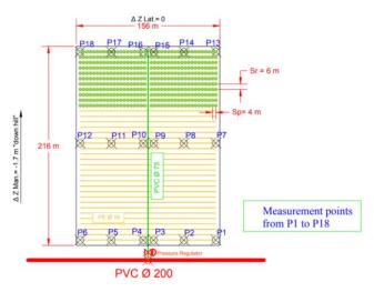
Fig. 11. The layout of the sub-unit (plot area);  $\Delta Z_{\text{Lat}} = \text{lateral}$  elevation difference (m),  $\Delta Z_{\text{Man}} = \text{Manifold elevation}$  difference (m), source: own elaboration
