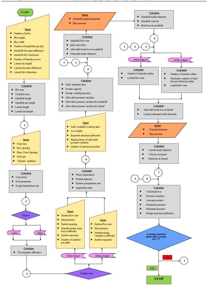
Fig. 1. Emission Uniformity on Sloping Surfaces (EUSS) model flow-chart; source: own elaboration
