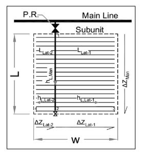
Fig. 5. Manifold design and layout; own elaboration; L = subunit length (m), W = subunit width (m), P.R. = pressure regulator,  $L_{\text{Lat}}$  = lateral length (m),  $h_{L, \text{Lat}}$  = the head loss in lateral (m),  $\Delta Z_{\text{Lat}}$  = lateral elevation difference (m),  $\Delta Z_{\text{Man}}$  = Manifold elevation difference (m); source: own elaboration
