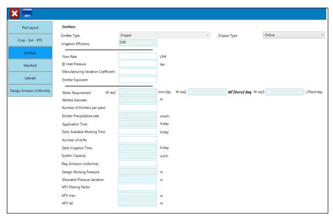
Fig. 4. Interface for emitters and the design parameter; source: own elaboration
