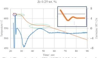
Fig. 4. Thermal analysis of F5 AlSi7Mg0.3Cu0.5 experimental alloy with the addition of 0.25 wt. % Zr
