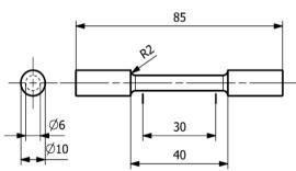
Fig. 3. Scheme of the testing sample (dimensions in mm)
