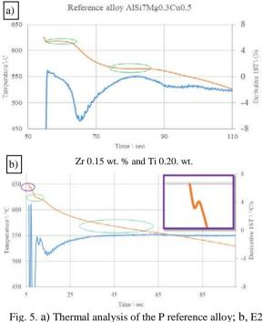
AlSi7Mg0.3Cu0.5Zr0.15 experimental alloy
