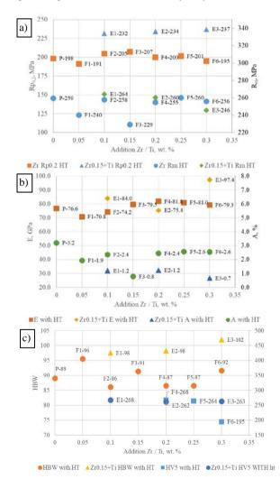
Fig. 6 Dependence of R<sub>m</sub>, Rp<sub>0,2</sub>, E, A, and HBW after heat treatment and HV5 Zr phases before heat treatment for P alloy and experimental F1- F6 and E1 - E3 alloys
