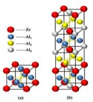
Fig. 2. Forms of the Al<sub>3</sub>Zr intermetallic phase precipitation in the crystallographic lattice: a) Ll<sub>2</sub> b) DO<sub>23</sub> [10]
