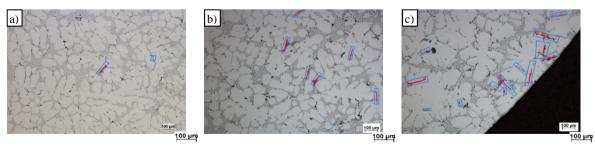
Fig. 8. Microstructure of primary and experimental alloys before HT a) R alloy, b) E1 alloy, c) E2 alloy, etchant H<sub>2</sub>SO<sub>4</sub>
