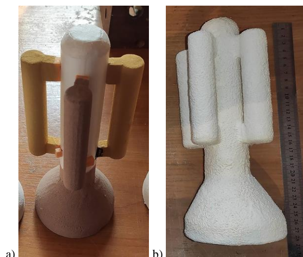
Fig. 1. Pattern with face coat (a) and ceramic shell mould (b)
