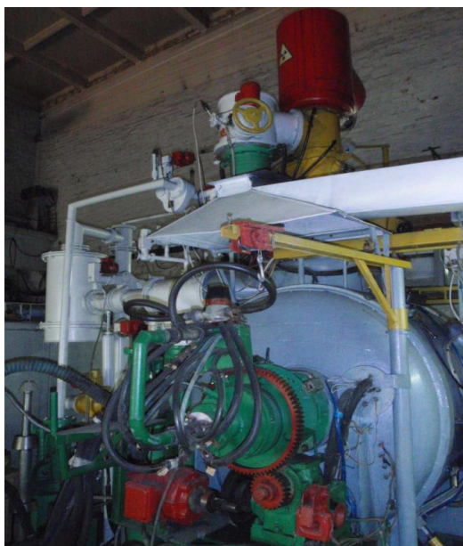
Fig. 2. Scheme and general view of the foundry EPLU-4: 1 - the movement mechanism of a cover; 2 - the mechanism of crucible rotation; 3 - crucible; 4 - vacuum chamber; 5 - electron-change gun
