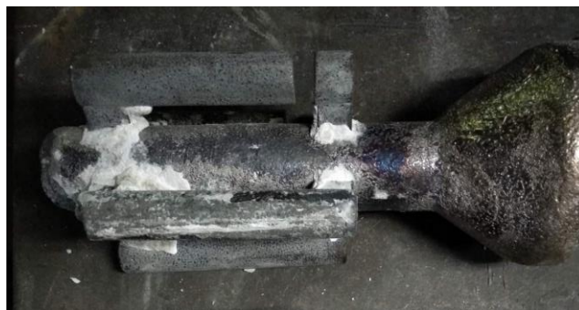
Fig. 3. Casting of CP titanium obtained in ceramic mold
