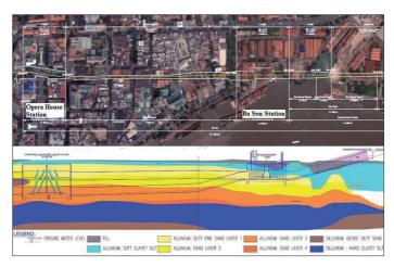
Fig.2 Subsoil condition of underground section
