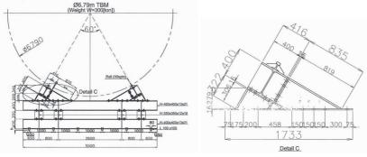
Fig. 7 Cross section of launching cradle
