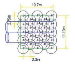
Fig. 4 Location and layout of jet grouting pile
