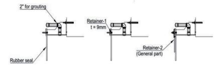
Fig. 9 Schematic diagram of Seal of soft eye
