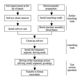
Fig.3 Process launching of Shield flow diagram
