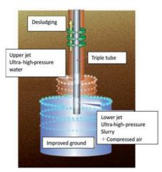
Fig.5 Schematic diagram of Jet grouting
