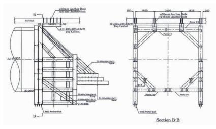
Fig. 8 Schematic diagram of thrust frame installation
