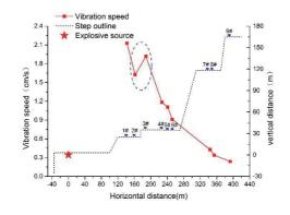
Figure 3. Vibration velocity of measuring point
