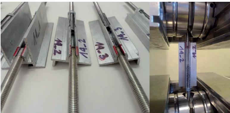
Fig. 13. Investigated bolt connections: a) view on specimens, b) clamped in a testing machine grips
