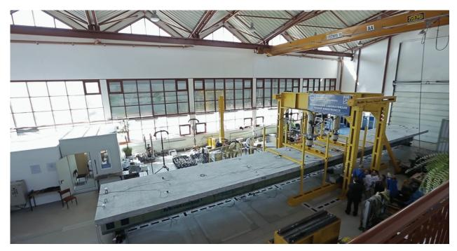
Fig. 3. Full scale laboratory tests of FRP road bridge at Rzeszow University of Technology [24]
