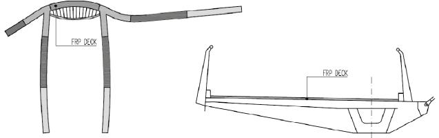
Fig. 14. View and cross section of the main span with FRP deck [6]
