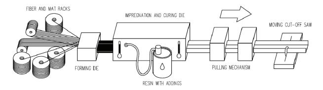
Fig. 2. Pultrusion process scheme [7]
