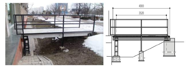
Fig. 6. Longitudinal section and photo of the footbridge [25]
