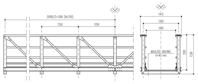
Fig. 5. Longitudinal and cross section of the pedestrian truss bridge [18]
