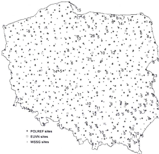
Fig. 8. Detected outlying WSSG height anomalies [cm] (numbers situated down left of the WSSG sites correspond to the outlying values of height anomalies)
