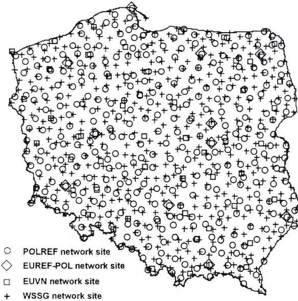
Fig. 1. Distribution of EUVN'97, EUREF-POL, POLREF and WSSG sites used for modelling quasigeoid
