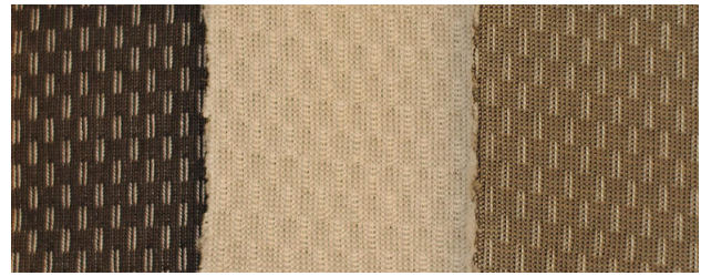
Fig. 6. Spacer fabric with interwoven optical fibres.
