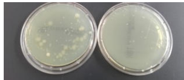
Fig. 18. Example of the comparison of the determination of the total amount of coliform bacteria (from the left) isolated from the control knitted fabric and irradiated under a 30-min exposure, lower part of the contact plate.
