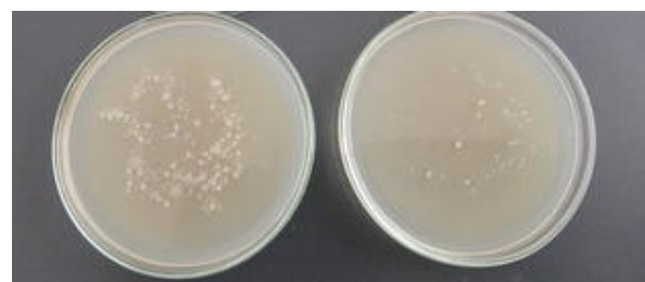
Fig. 20. Example of a comparison of the determination of the total number of actinomycetes (from the left) isolated from the control knitted fabric and irradiated under a 30-min exposure, lower part of the contact plate.
