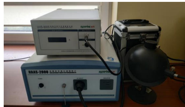
Fig. 2. Measurement station: HAAS-2000 spectroradiometer, UVS-8005 power supply, Ulbricht sphere.
