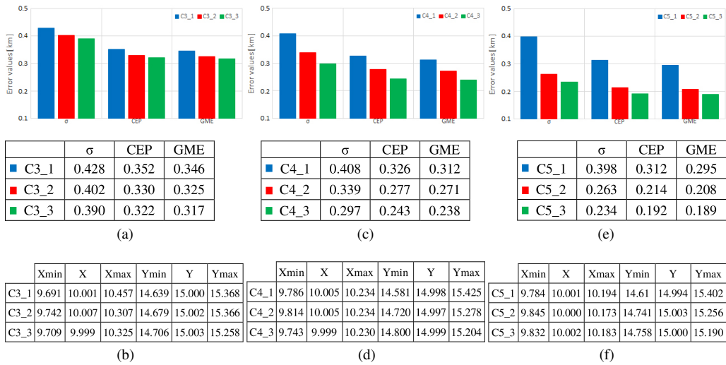
Fig. 11. Estimation of emitter location errors ( \sigma , CEP and GME) located in tested point (10, 15) [km] for all configurations of DFs deployment (100 generated bearings realizations, accuracy of bearing error measurement \xi = 1^\circ ): (a–b) variants for 3 DFs; (c–d) variants for 4 DFs; (e–f) variants for 5 DFs.
