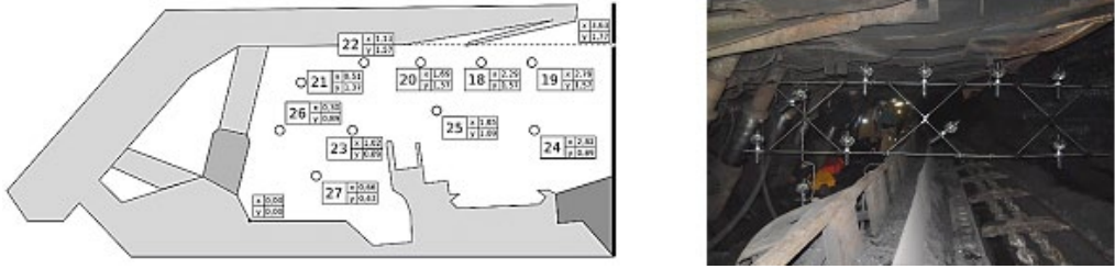
Fig. 16. Measuring cross-section, longwall Z-11, face end. Section No 99/119
