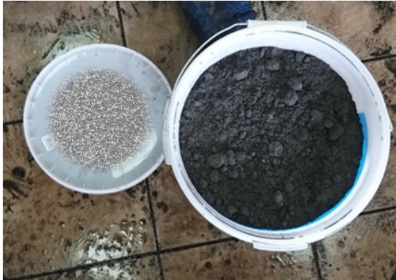
Fig. 1. Raw coal burning waste for testing
