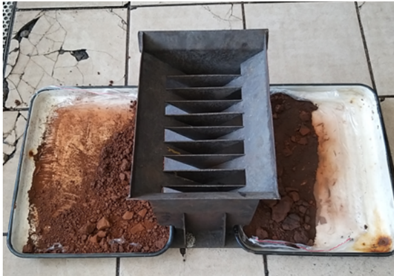
Fig. 2. Classification of the material using the sample divider
