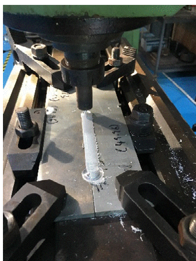
Fig. 2. Workpiece clamped onto the machine table
