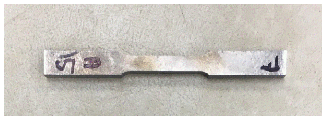
Fig. 4. Tensile test sample
