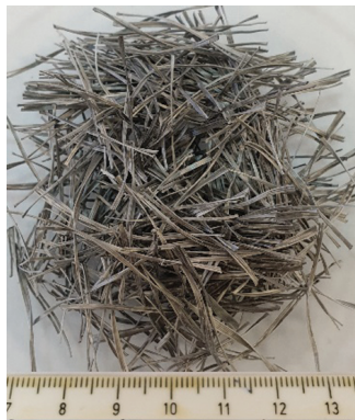
Fig. 3. Polymer fibers of a length of 24 mm
