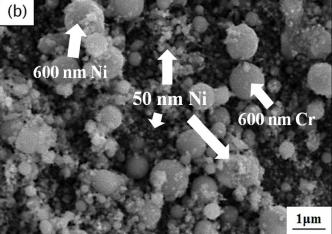
Fig. 1. SEM photographs of the surface morphology (a) nNi powders, and (b) 30% nNi specimen after 1 h ball mixing
