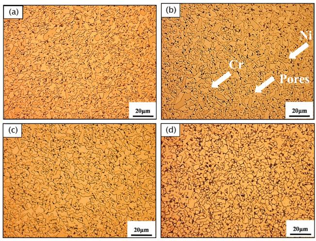
Fig. 4. OM morphologic observations of hot-pressed Cr-50 mass% Ni alloys by adding different amounts of nNi powders (a) 0, (b) 10, (c) 20, and (d) 30 mass%
