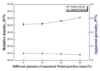
Fig. 3. Comparison of the relative density and apparent porosity of hot-pressed Cr-50 mass% Ni alloys by adding different amounts of nNi powders
