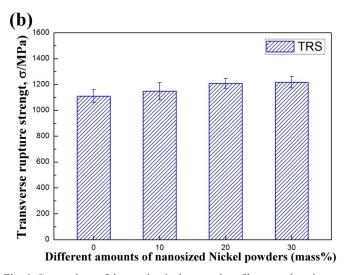
Fig. 6. Comparison of the mechanical properties of hot pressing sintering Cr-50 mass% Ni alloys by adding different amounts of nanosized nickel powders (a) hardness, and (b) TRS tests
