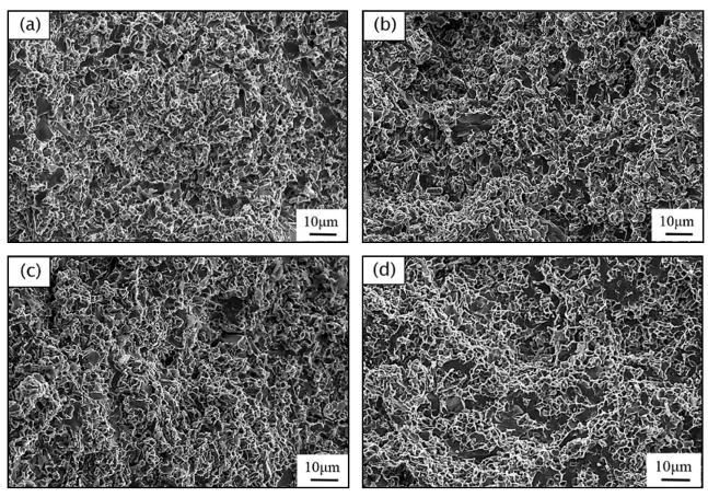
Fig. 7. Fractographic observation of hot-pressed Cr-50 mass% Ni alloys by adding different amounts of nNi powders (a) 0, (b) 10, (c) 20, and (d) 30 mass%
