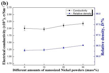
Fig. 5. Comparison of the properties of hot-pressed Cr-50 mass% Ni alloys by adding different amounts of nNi powders (a) interface numbers and grain size, and (b) electrical conductivity and relative density
