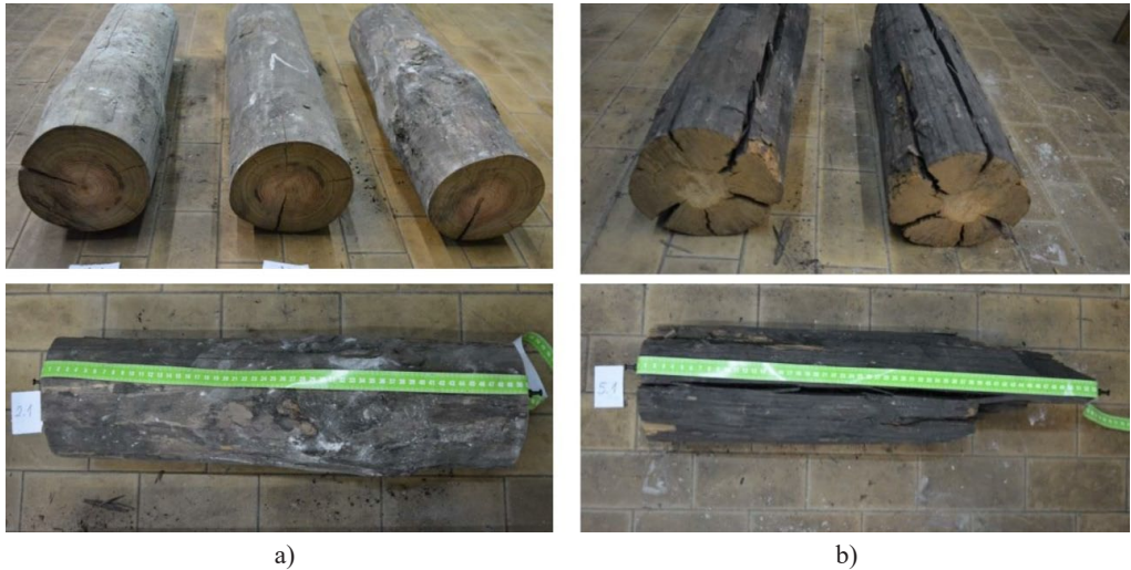
Fig. 3. A view of examples of fragments cut out from the props and roof-bars from groups: a) 2, b) 5
