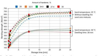
Fig. 7. The combined effect of the increased sand temperature and dwelling time on the hardening characteristic of the warm-box sand cores
