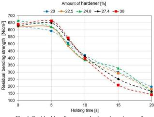
Fig. 6. Residual bending strength of sand specimens after thermal exposure
