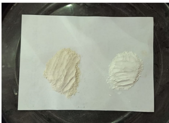
Fig. 18. Photograph showing the difference in whiteness before and after magnetic separation
