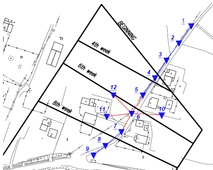
Fig. 3. Location of the points of the field rosette and the progress of the operational front in time ( Source: own study based on materials from the Marcel Coal Mine )
