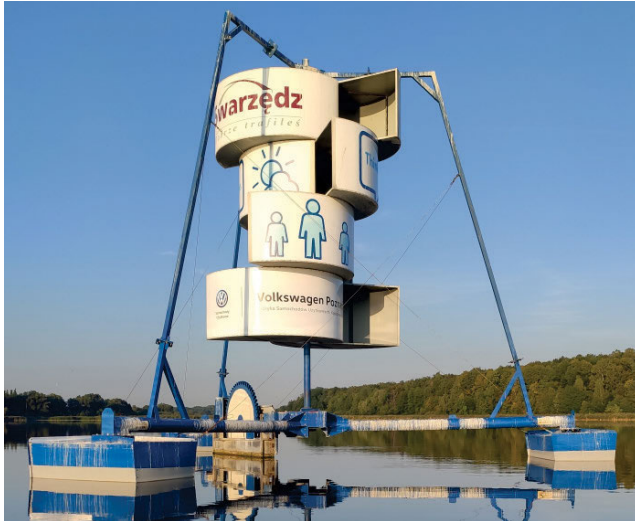
Photo 1. Wind driven pulverising aerator located on Lake Swarzędzkie (phot.: A. Osuch)
