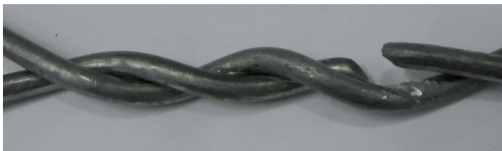
Fig. 9. Double twist after failure
