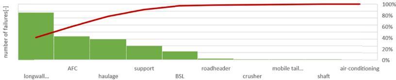
Fig. 10. Pareto chart for the number of mechanical failures in shearer longwalls
