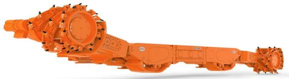
Fig. 2. Mechanised shearer complex ([www.lw.com.pl](http://www.lw.com.pl)), JOY 7LS0 mechanised longwall shearer (<https://mining.komatsu/>)
