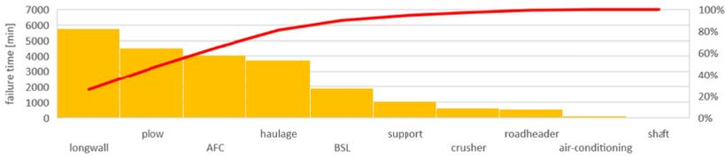
Fig. 17. Pareto chart for the duration of electrical failures in plow longwalls
