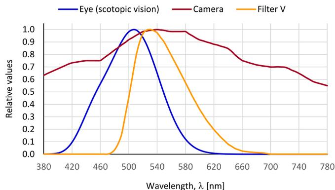
**Fig. 5.** Spectral characteristic of the fully dark-adapted human eye (scotopic vision), the V filter of the Johnson–Cousins photometric system, and the selected CCD camera. See the text for more details
