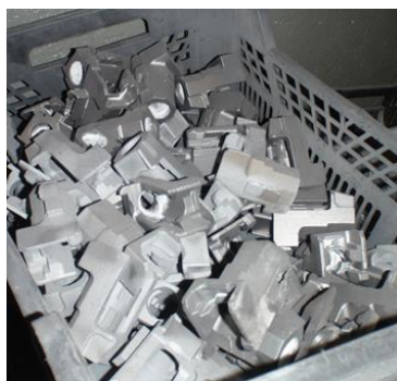
Fig. 1. Steel castings produced by investment casting
