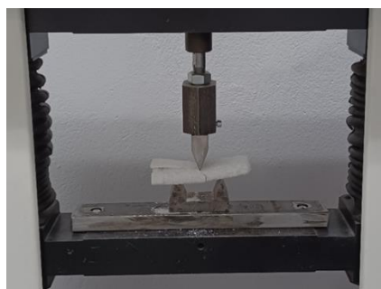
Fig. 5. Investigations of bending strength
