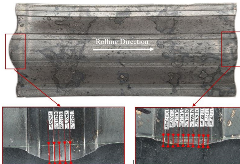
Fig. 20. The obtained strip with example measurements of the difference in elongation: A – the end of the strip, B – the beginning of the strip
