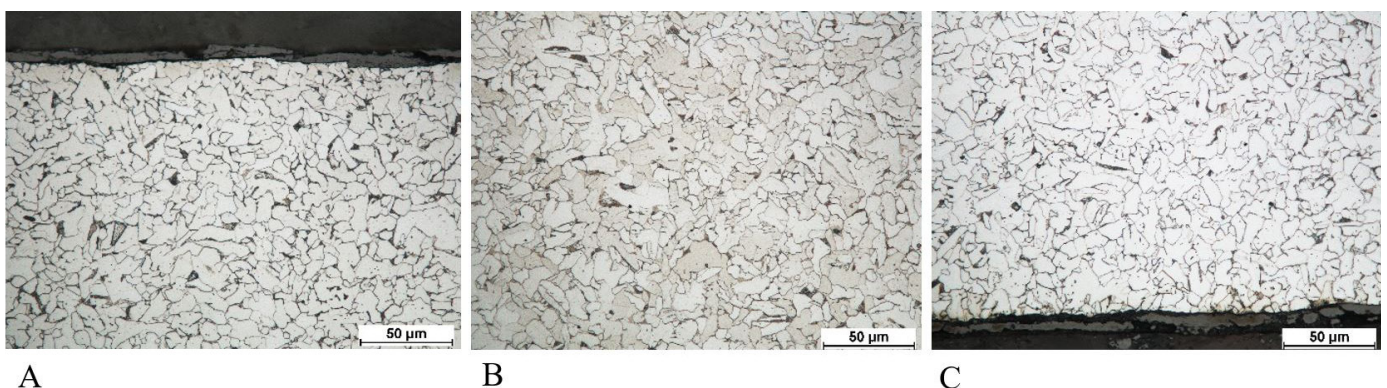
Fig. 6. Images of material microstructure under delivery conditions for transverse surfaces: A – microstructure at the top surface, B – microstructure inside the material, C – microstructure at the bottom surface
