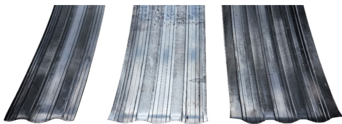
Fig. 7. Strips obtained after rolling. From left: 56, 80 and 92 mm strips
