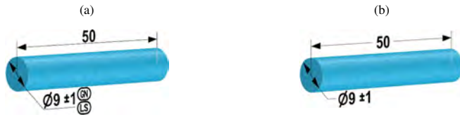
Fig. 16. (a) Shaft with limit dimensions specified according to the ISO GPS system that defines identical requirements as the default ASME specification; (b) ASME specification. [authors' drawing]
