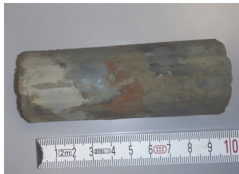
Fig. 2. Sample for UU test from the core extracted from 9–9.5 m
