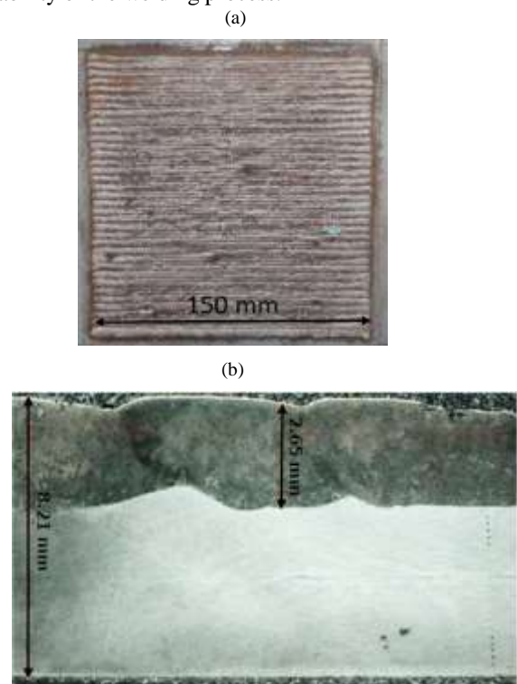
Fig.1. (a) HC-O hard-face plate produced by an automatized arc-welding process performed by an H-Frame welding machine, (b) fragment of the cross-section.
