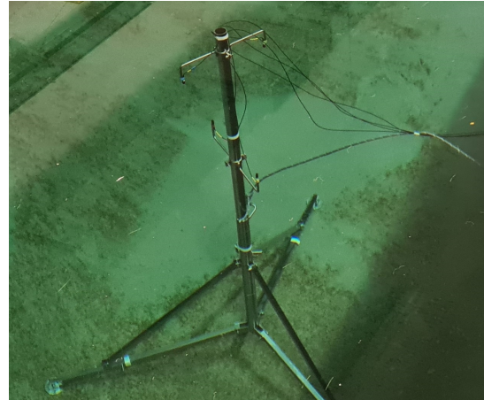
Fig. 5. Submerged mast with the receiving transducers
