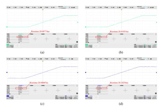
Fig. 19. (a) Traditional DDS 20.00774 ns rise time, (b) traditional DDS 20.45953 ns rise time, (c) mapping method 20.08007 ns rise time, (d) mapping method 20.18256 ns rise time.
