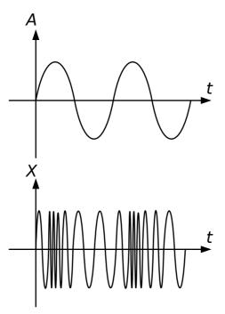
Fig. 11. Frequency modulation diagram.
