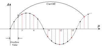
Fig. 3. Diagram of the phase overflow.
