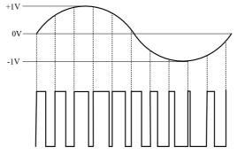
Fig. 12. Schematic diagram of the PWM waveform.
