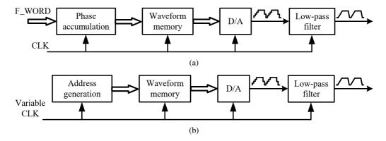
Fig. 1. (a) DDFS architecture, (b) DDWS architecture.
