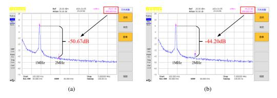
Fig. 18. (a) Waveform synthesis based on phase-amplitude mapping, (b) traditional DDS.
