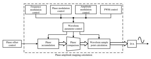
Fig. 8. Block diagram of the phase-amplitude mapping based waveform modulation principle.
