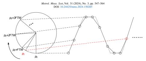
Fig. 6. Schematic of pulse waveform with the non-integer multiple sampling rate.
