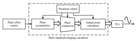
Fig. 7. Block diagram of the pulse waveform synthesis principle.
