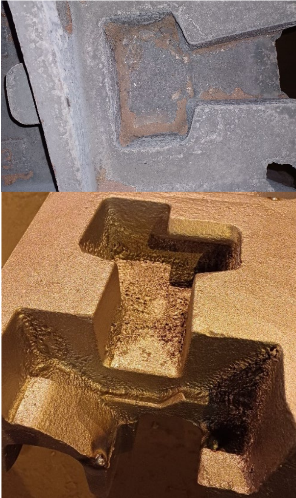
Fig. 3. A view of cast steel casting defects, i.e. burn-on of moulding sand based on chromite prepared in Alphasert technology in the case of a profile of a mining chain conveyor (net mass 415 kg) cast from unalloyed cast steel in Huta Małapanew Sp. z o.o.
