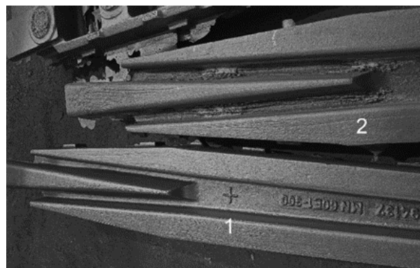
Fig. 1. A view of the running part of Insert R300 frog (net mass 273 kg) cast from manganese cast steel in Huta Małapanew Sp. z o.o. 1 – when moulding sand based on chromite sand in Alphaset technology was used; 2 – when sand based on quartz sand in Alphaset technology was used
