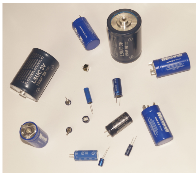
Fig. 3. Examples of supercapacitors under tests at the Warsaw University of Technology
